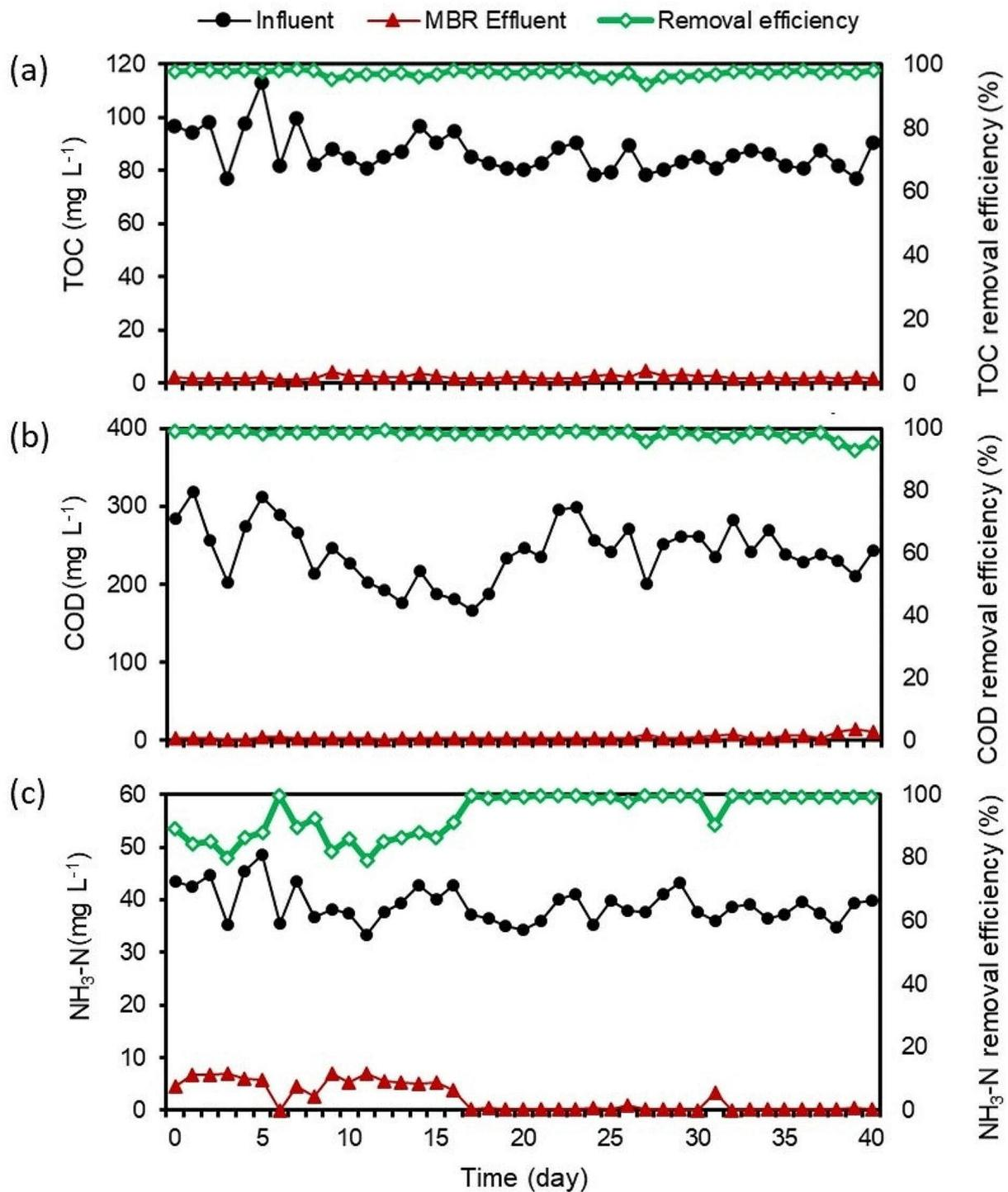
**Fig. 2** Long-term stability performance of MBR system as recorded in influent and effluent concentration and removal efficiency: (a) TOC, (b) COD, and (c) NH<sub>3</sub>-N
