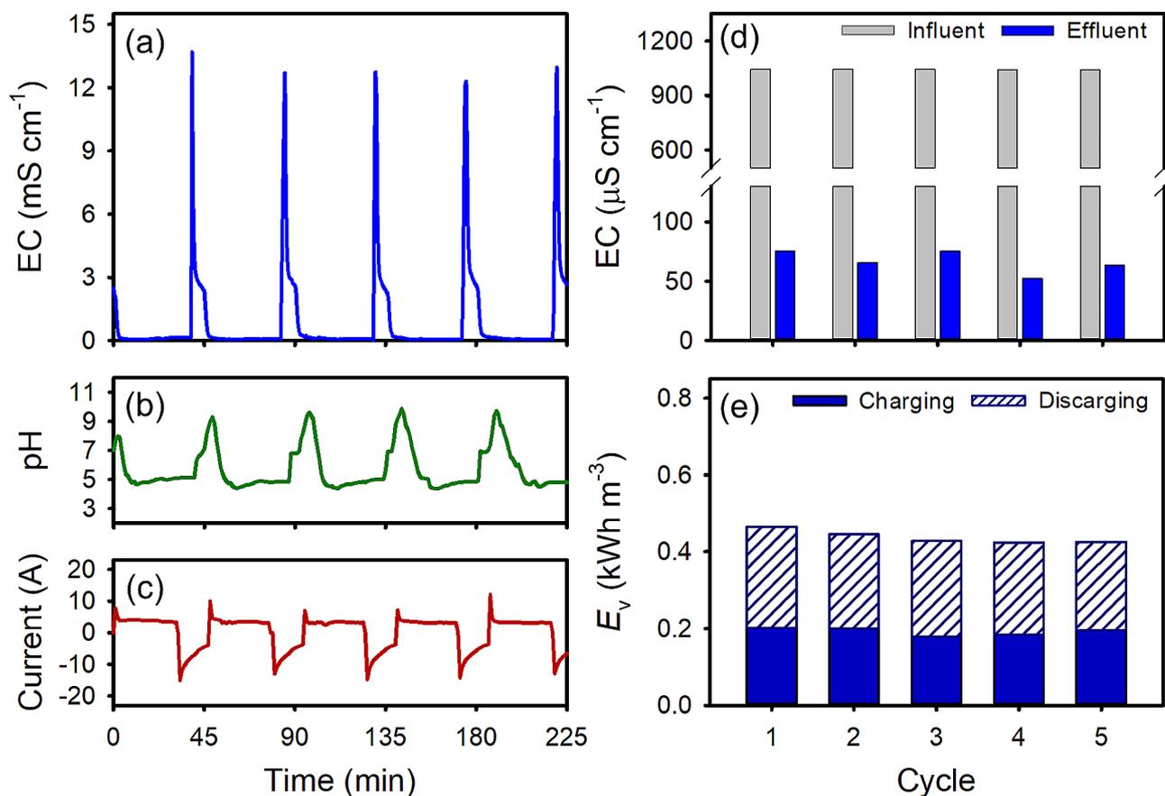
**Fig. 6** System performance of MCDI experiment over 5 repeated cycles under optimal operation condition. **(a)** EC, **(b)** pH, and **(c)** current profile for 5-cycle operation. **(d)** EC of influent and effluent, and **(e)**  $E_v$  of charging and discharging step for MCDI system
