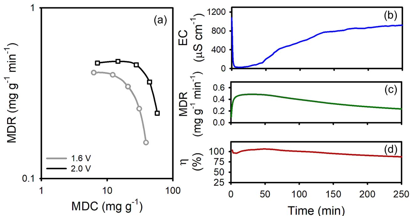
**Fig. 4** (a) Variation of CDI Ragone plots according to the applied voltage and performances of MCDI system using MBR effluent at 2.0 V with flow rate of 350 mL min<sup>-1</sup>: (b) EC, (c) MDR, and (d)  $\eta$
