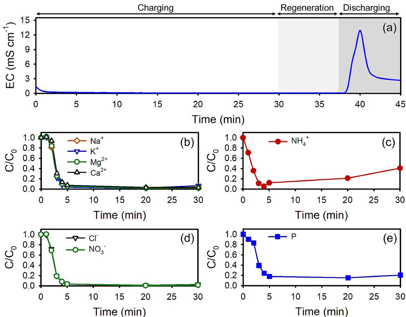
**Fig. 5** MCDI system performance under optimal operation condition (2.0 V for 30 min in charging step, 0.0 V for 3.75 min followed by  $-2.0$  V for 3.75 min in stop-flow regeneration step, and  $-2.0$  V for 7.5 min in discharging step). Variations in (a) EC, (b)  $\text{Na}^+$ ,  $\text{K}^+$ ,  $\text{Ca}^{2+}$ , and  $\text{Mg}^{2+}$ , (c)  $\text{NH}_4^+$ , (d)  $\text{Cl}^-$  and  $\text{NO}_3^-$ , and (e) total P measured as phosphate ions
