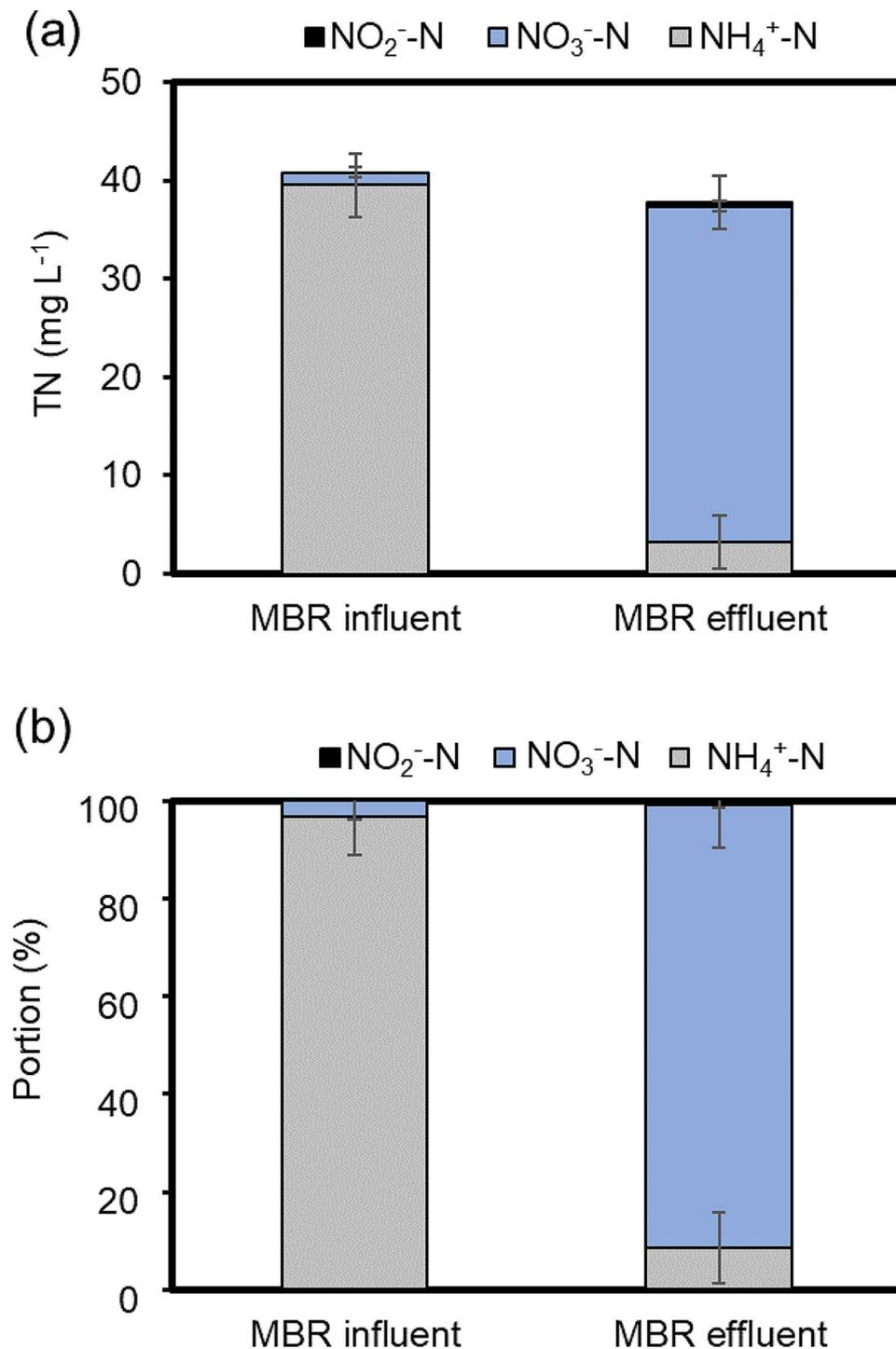
**Fig. 3** (a) Distribution and (b) portion of N species in both the influent and effluent of the MBR
